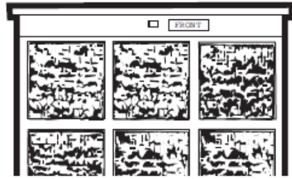
Dirty filter—Needs cleaning
