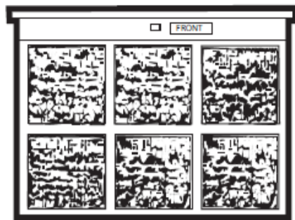
Dirty filter— Needs cleaning
