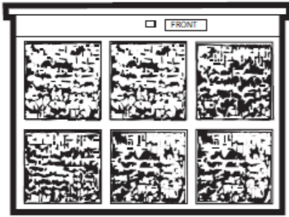
Dirty filter— Needs cleaning
